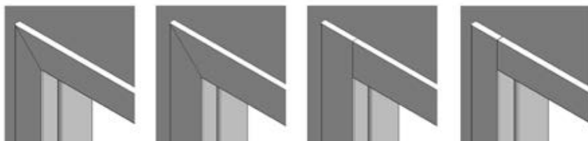
version A joint angle 45° width 60 mm without extra charge
