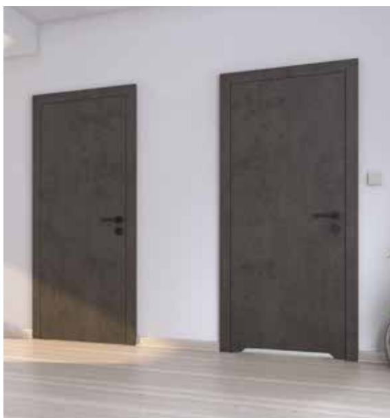
door leaf in the REVES system (on the left), right - opening inward; door leaf in the DUO system (on the right), left - opening outward
